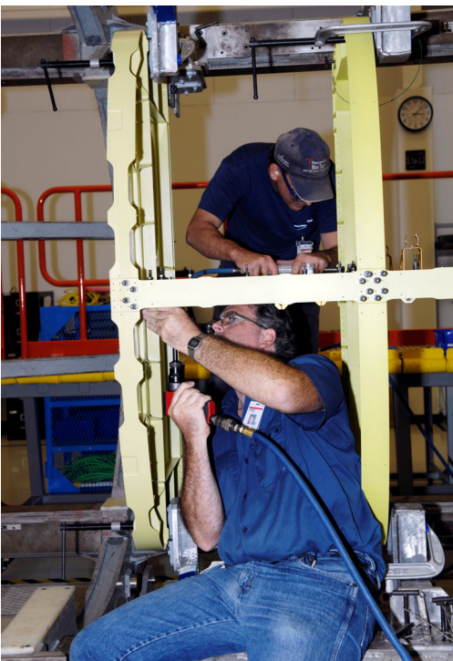
Workers Mark Reed (top) and Jessie Kemp drill holes on an RQ-4 at Northrop Grumman Unmanned Systems Center in Moss Point. Northrop Grumman photo
